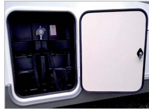
Fig.6.30 - Gas cylinder compartment
